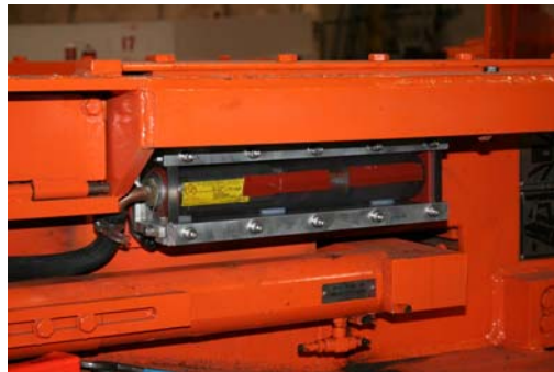
Figure 5 - Geosteering Field Generator
